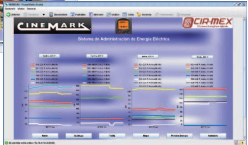
To make data management easier, a series of screens were programmed in PowerStudio Scada which help to manage information such as energy indexes, billing simulation, graphics, etc.
